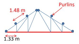
Weight of roof covering sheeting =  $150 \times 1.48 = 222 \text{ N/m}$
