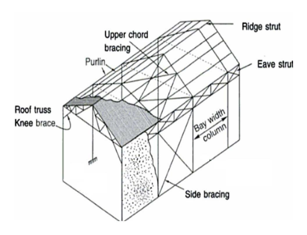
Load on roof truss:- DL, LL, WL/SL
